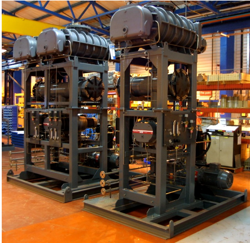
Fig. 6. Two-part dry mechanical vacuum pump system manufactured for a multi-chamber titanium refining plant including two ISM furnaces
